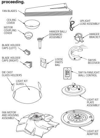
IMPORTANT: Your ceiling fan is supplied with an SW116 Fan/Light Wall Control (transmitter) and a remote control SW105 Receiver which mounts under the ceiling cover. This system allows you to regulate your ceiling fan speed, airflow direction, and light intensity. An optional Emerson Electric SR110 Remote Control may also be used.
